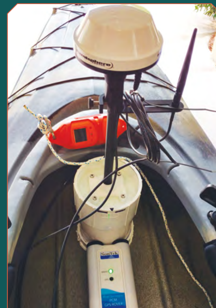
The PVC sleeve contains a SonTek M9, used to survey the lake bottom; the orange SonTek CastAway provided quick conductivity, temperature and depth data for correcting sound-speed variations.
